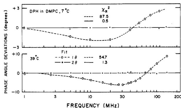
FIGURE 6: Deviations between the measured and calculated differential phase angles for DPH in DMPC vesicles. Deviations are shown for the two correlation time model with  $r_\infty = 0$  (●) and for the single correlation time model (○).
