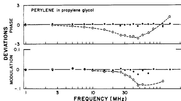
FIGURE 3: Deviation between the measured and calculated data for perylene in propylene glycol at -9 °C. Deviations are shown for the best fits obtained by using a single correlation time (○) and two correlation times (●). In both cases  $r_0$  was held constant at the measured value of 0.312.
