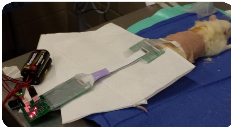
Figure 13. Mounting the Sensor Array to the Wound
