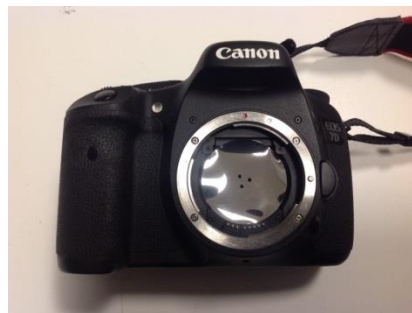
Figure 38. Aperture Mask Positioned on the Camera
