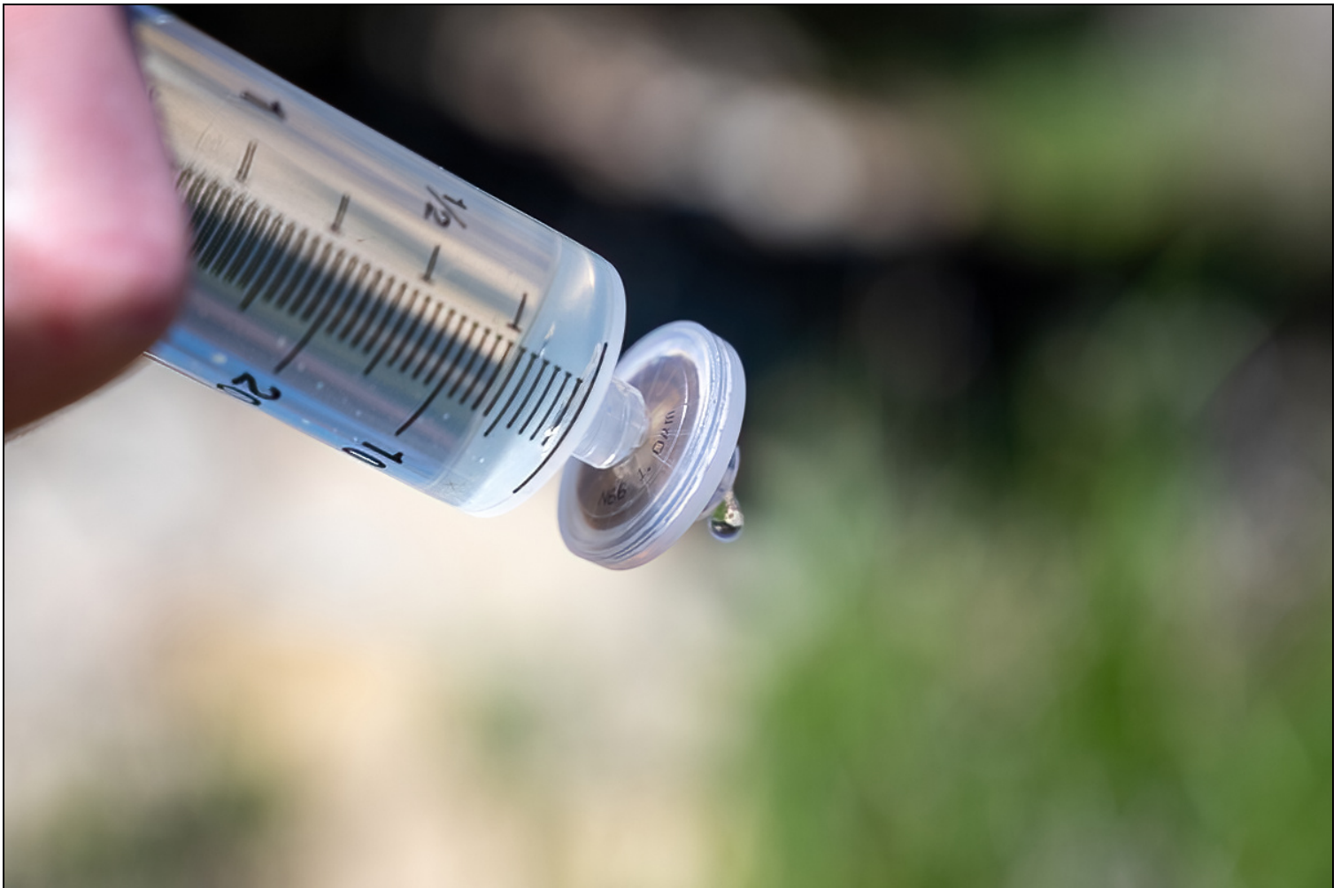
UCSB student Mckenzie Goetz filters water through 1 um filter to obtain an eDNA sample.
