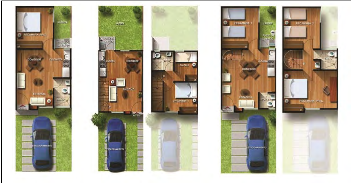
Figure 4.10 Typical housing unit floor plans
