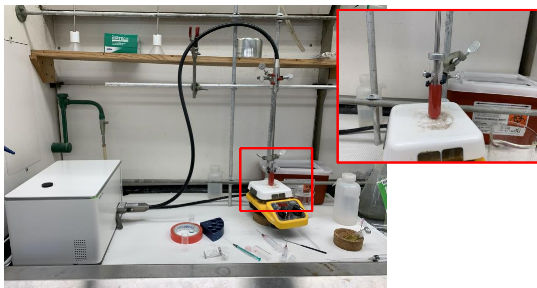
Figure 2.24. Example of ReactIR setup used for kinetic analysis.
