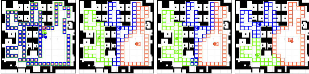
Figure 4.5: Snapshots from a simulation of three robots partitioning an environment with black obstacles using the \mathcal{H}_{\min, \inf} One-to-base station algorithm. Note that the initial condition is the same as in Figure 4.4, but the evolution is different.
