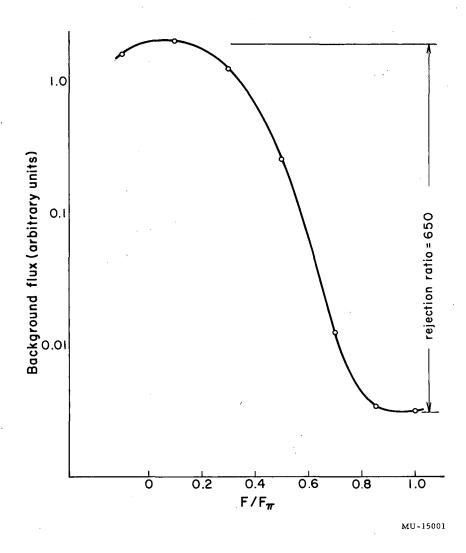
Fig. 6. Background flux vs  $F/F_{\pi}$  behind final collimator (1-in. vertical by 0.5-in. horizontal uranium-jawed slit). Collimator ahead of Q2 3.5 in. in diameter. Brass rod 0.75 in. in diam was installed on Q2 axis. V = 250 ky constant; H varied.
