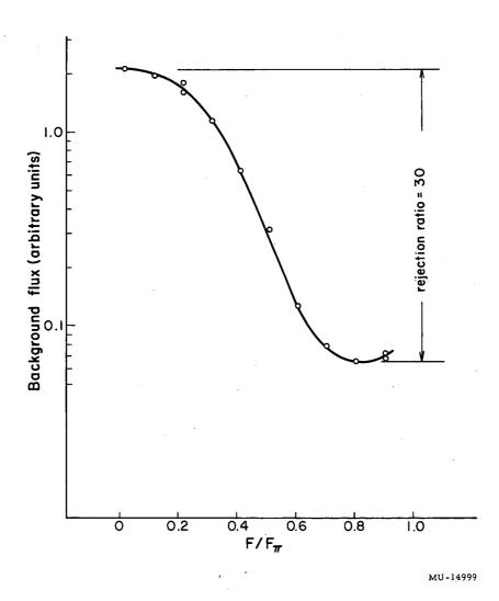
Fig. 5. Background flux vs  $F/F_{\pi}$  taken directly behind 3-in. - diam collimator ahead of Q2. V = 240 kv constant; H varied.
