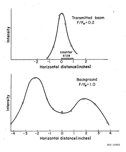
Fig. 7. Horizontal profiles of transmitted beam and of back-ground 5 ft behind bubble chamber. Q2 was focused at this point with no final collimator. Rejection ratio with 1-in.-diameter counter was 1500.
