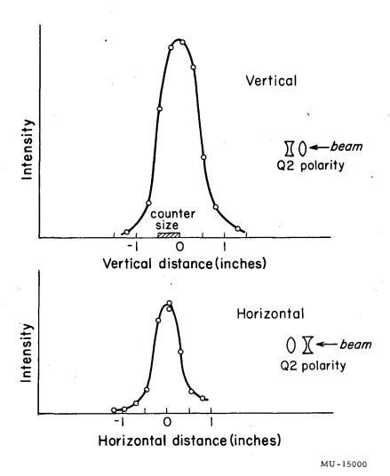
Fig. 9. Vertical and horizontal beam profiles at focus of Q2 (position of final collimator). F/F $_{\pi}$  = 0.2. Total flux integrated over 1-in. vertical by 0.5-in. horizontal central area was 11 x 10<sup>3</sup>  $\pi/10^{10}$  protons on target.
