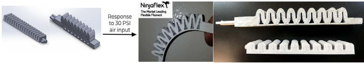
Figure 4. Response of Pneunets bending actuator to 30psi air input (left). Air leaks in the 3d printed actuator (right).
