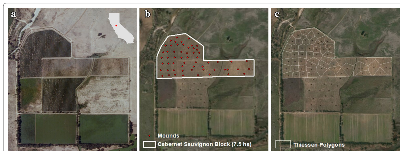
Fig. 1 Study vineyard in southern Sacramento County, California, USA. The vineyard prior to removal is shown in a . The boundaries of the Cabernet Sauvignon plot are outlined in b with dots representing woody debris mounds resulting from uprooted vines. The Thiessen polygons around mounds in c were used to estimate source area for C per hectare estimates
