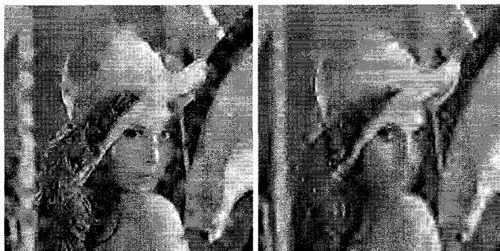
Figure 2. Images displayed here show the visual effects of loss for the hybrid coder (left) vs. the SPIHT+RCPC/CRC coder (right) at equal distortion ( PSNR = 23.5dB ).
