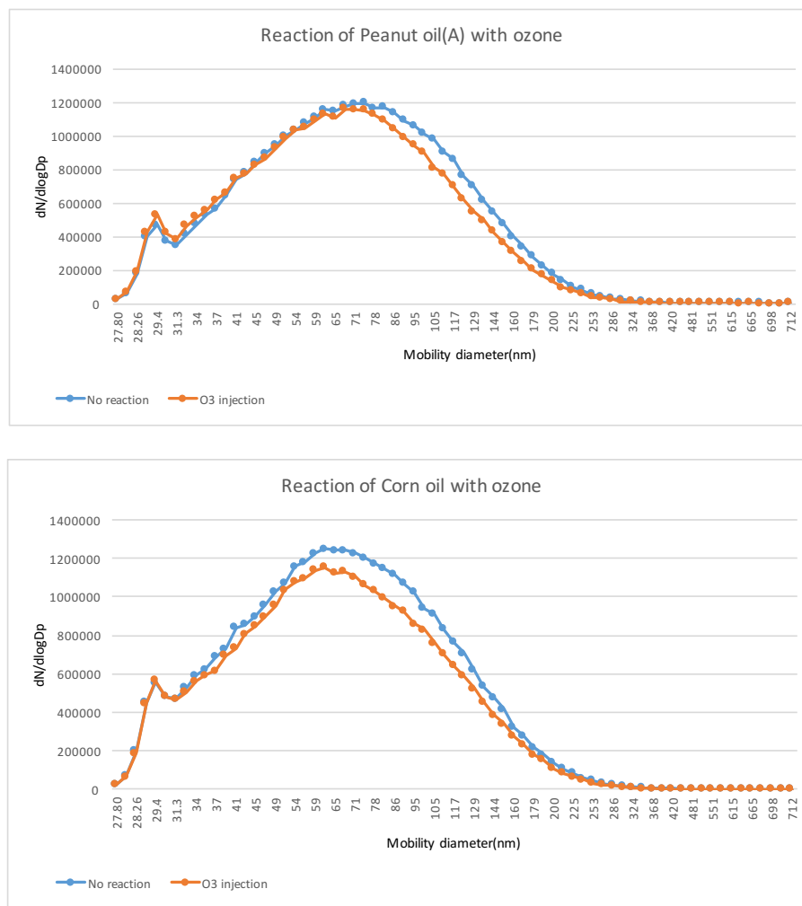
Fig.11 Examples of particle size distribution: (a) peanut oil reaction with ozone and (b) corn oil reaction with ozone.
