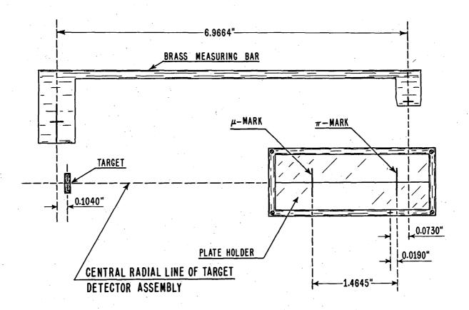
Fig. 11 Linear measurements of target-detector assembly taken during Run I. The measurements were obtained with the aid of a low-power microscope attached to a micrometer traveling in a direction parallel to that of the median line.
