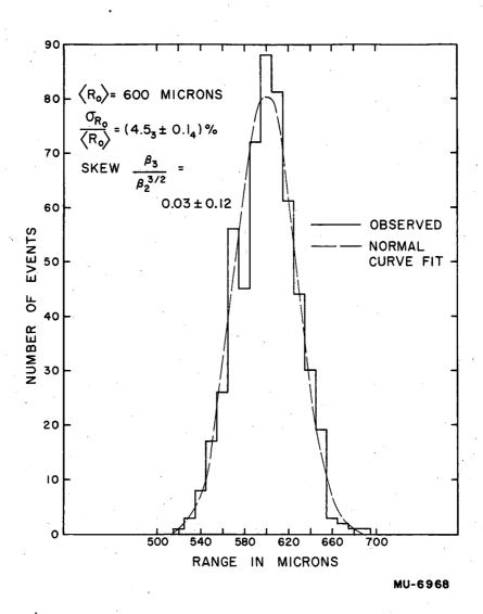
Fig. 13 Distribution of ranges of mu-completes: 558 events are taken from 12 plates and normalized to a mean range of 600 microns. A normal curve fit to the experimental data gives a  $\chi^2$ -test significance level of  $\approx$  0.4.
