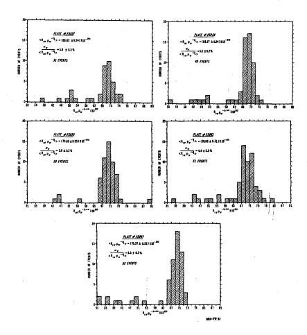
Fig. 14 Pion normalized-range distributions from the 5 plates of Run I. Note the small amount of background. Percentage variance slightly but not significantly lower than predicted value ( $R_{l\pi}$  in units of microns, and  $p_{\pi}$  in gauss-mm.)
