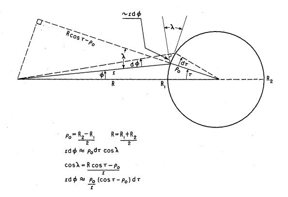
Fig. 2. Circular approximation to orbit in median plane followed by a charged particle. This figure gives an approximate geometrical relation necessary in the calculation of the momentum of the particle.
