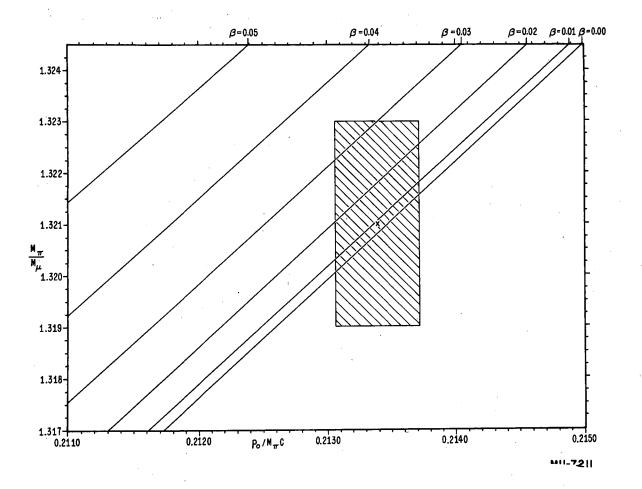
Fig. 20 Graphical solution to estimate of neutrino mass from Eq. 6.3. This essentially is an enlarged plot of Fig. 6. The hatched region represents the area subtended by the probable errors in the  $\pi/\mu$  mass ratio and the quantity  $p_0/m_\pi c$ . A probable upper limit of 6 to 7  $m_0$  is indicated.  $(\beta = m_V/m_\mu)$
