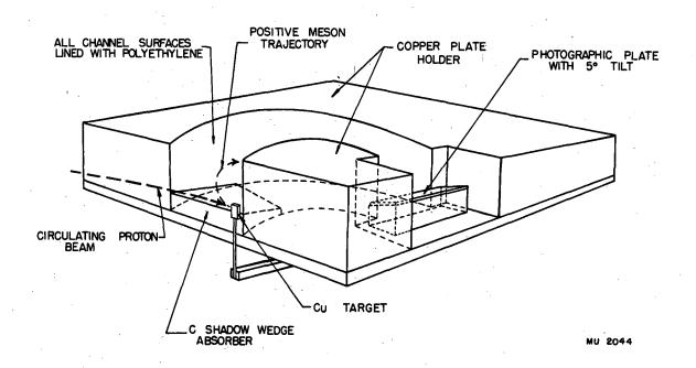
Fig. 8 Perspective view of the experimental apparatus of Run I; the target and detector assembly are rigidly mounted on a dural plate which is fixed in position on the proton probe cart.
