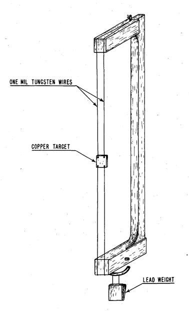
Fig. 9 Full-scale drawing of improved target holder of Run II.
