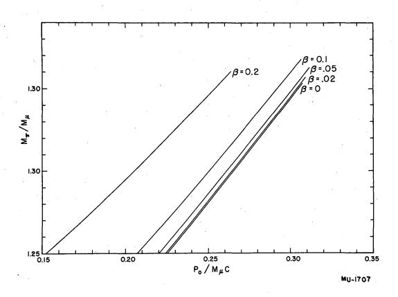
Fig. 6 The relation between the  $\pi$ - and  $\mu$ -masses for various values of the neutral-particle mass  $\nu$  as a function of the absolute decay momentum of the  $\mu$ -meson. This family of curves shows the extreme sensitivity of the derived neutrino mass to slight variations of the  $\pi/\mu$  mass ratio and the quantity  $p_0/m_\mu c$ .
