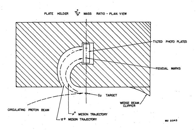
Fig. 7 Plan view of the experimental arrangement (Run I) inside the vacuum tank of the cyclotron. Typical pion and muon orbits are shown leaving the target and entering the emulsion detector.
