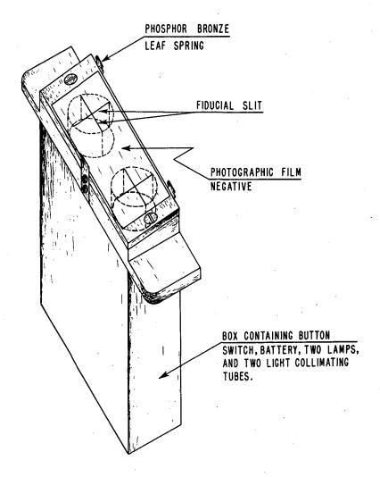
Fig. 10. Isometric full-scale sketch of plate holder. Fiducial slits were obtained by photographing a drawing of two sets of mutually perpendicular lines. The negative of this photograph is glass-backed and is cemented to the inclined brass surface. The nuclear emulsion detector is fixed in place on top of the film negative with the aid of the phosphor bronze leaf springs. A latent image of the fiducial lines is formed in the emulsion just prior to exposure within the cyclotron.
