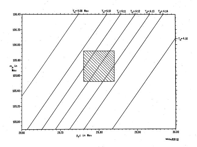
Fig. 19 Graphical solution to value of the absolute decay kinetic energy of the muon from the relativistic relation,
