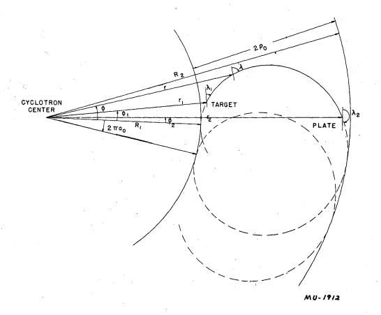
Fig. 1. Diagram illustrating the trochoidal type of orbit in the median plane followed by a charged particle in the radially decreasing magnetic field of the cyclotron.
