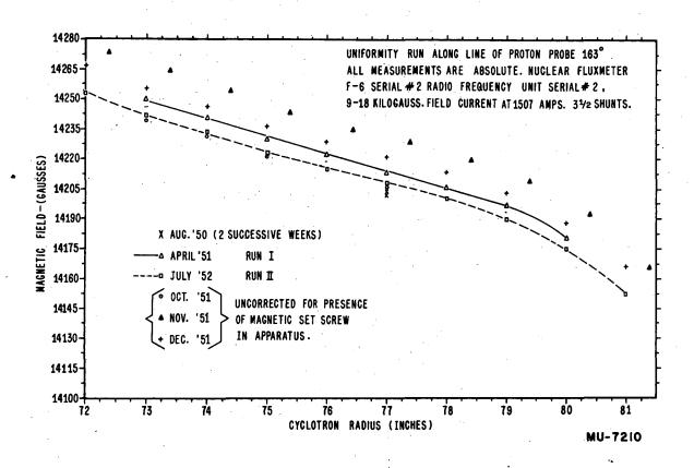
Fig. 12 Absolute measurements of the cyclotron magnetic field taken with the nuclear fluxmeter. Note the change in slope in the neighborhood of 80 inches.
