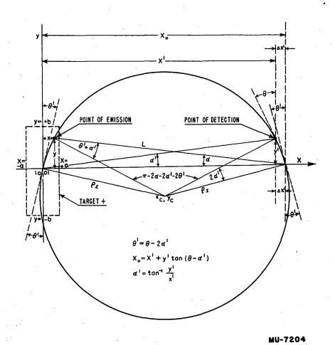
Fig. 3. Circular approximation to trajectory of meson leaving target at point (x, y) and entering detector at point (x', y'). This diagram shows all the pertinent geometrical parameters and relations required for the corrections to the momentum calculation owing to the finite size of the target and the finite area of the detector.
