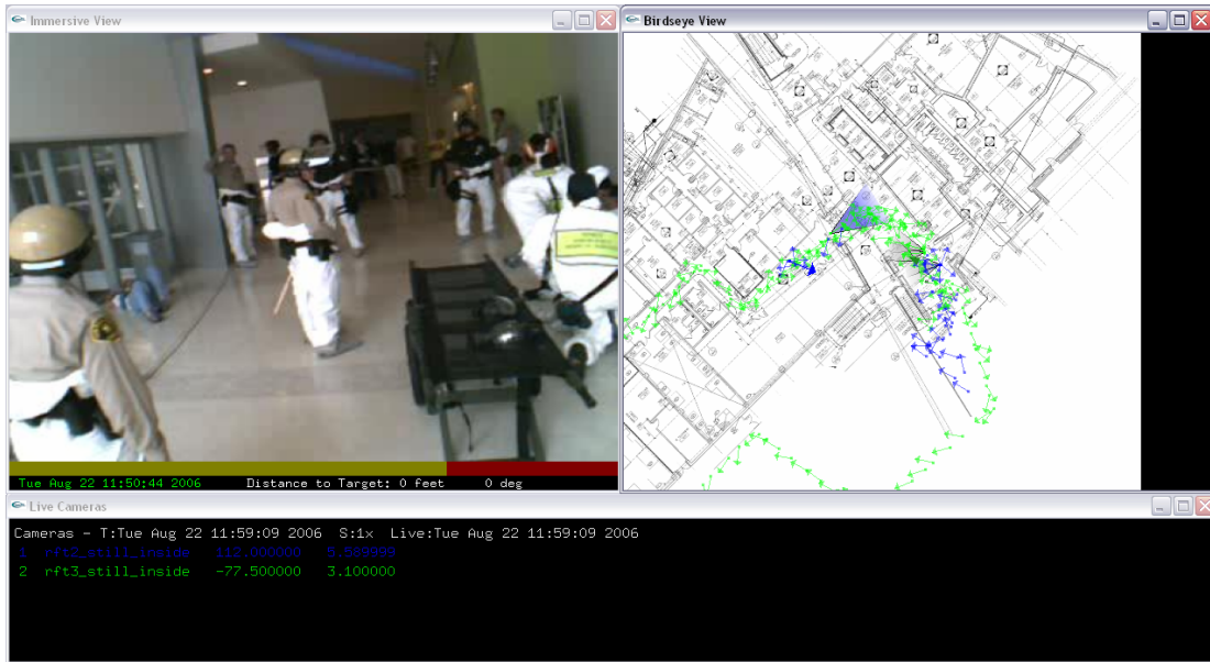
Figure 1.1: A screenshot of a typical RealityFlythrough session. The left window is the immersive view that shows the video feeds, camera images, or transitions. The right window is the birdseye view that shows all of the images that can be viewed. Each arrow represents a camera view, and the arrows are colored to indicate which camera they came from. The bottom window provides some information about the current state of the system.
