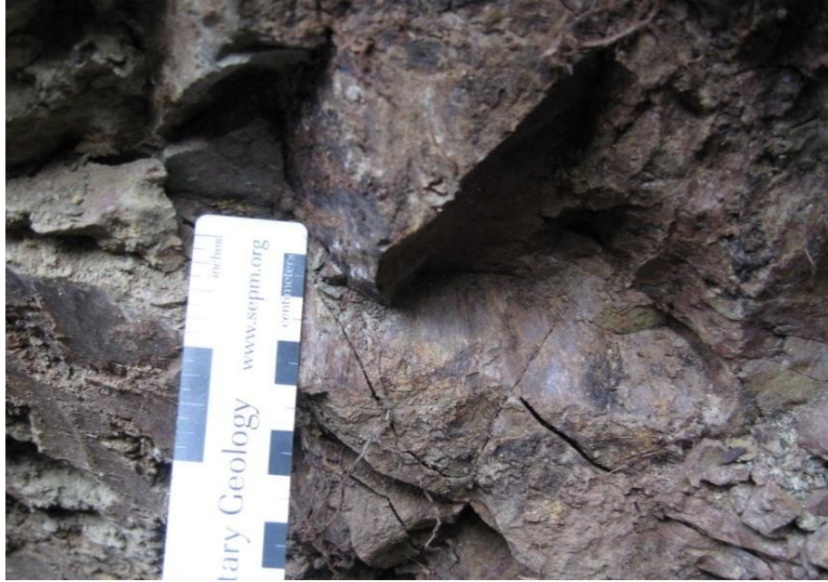
Figure 3-60. Scaly cleavage observed in dark-red mudstone, showing fine slickenside on cleavage plane
