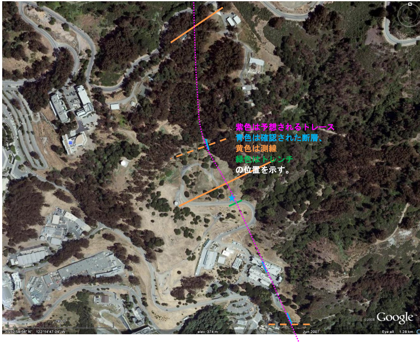
Figure A-1. Initial planned locations of geophysical survey lines and a trench.
