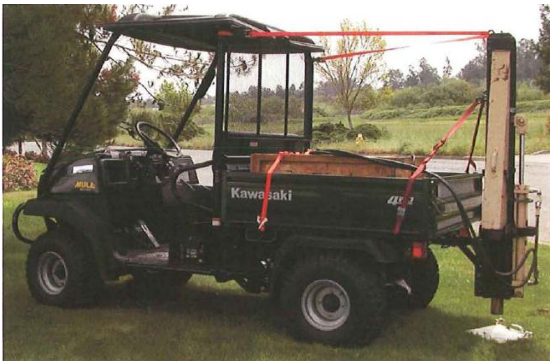
Figure 3-32. Accelerated weight drop system mounted on an ATV (Black, 2009).
