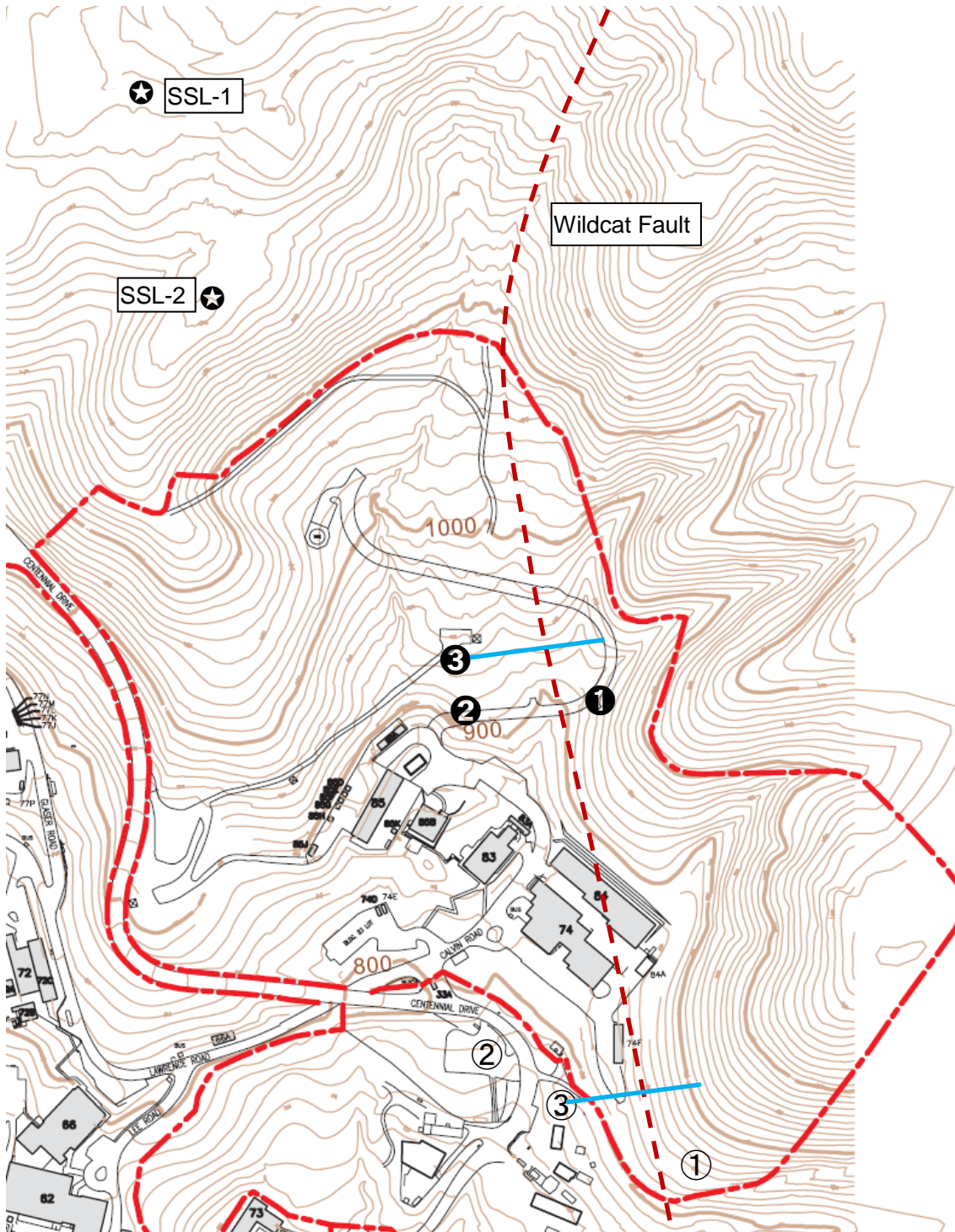
Figure 3-83. Potential borehole locations and existing deep boreholes SSL-1 and SSL-2 in relation to the Wildcat Fault.
