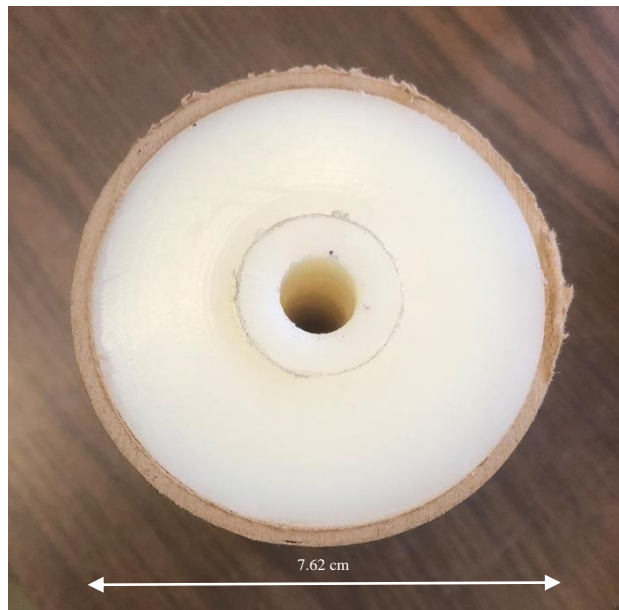
Figure 4.8. Top view of nylon 6 fuel grain inserted into sleeve.
