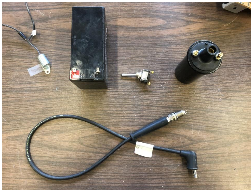
Figure 4.9. Isolated spark plug assembly components.
