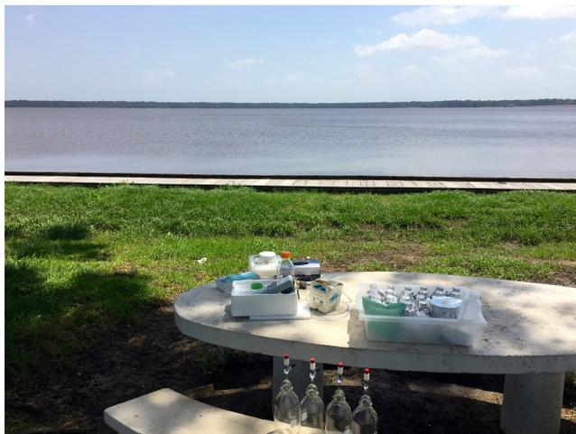
**Figure 2.6:** Sampling at Lake Houston. Pictured are the location of water sampling, flasks and Wheaton Bottles.
