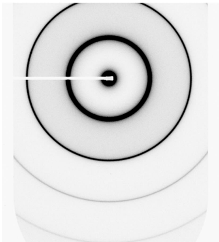
Figure 2.6 Powder diffraction ring pattern of DPPC membranes.
