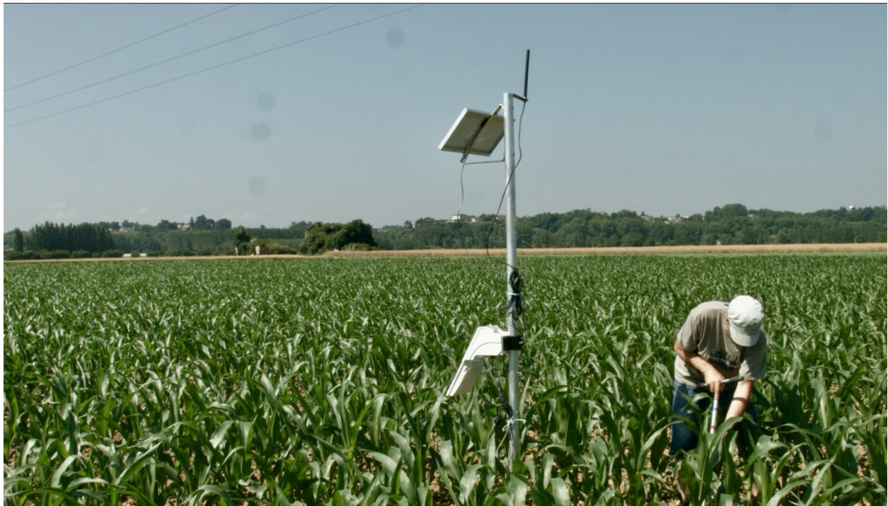
Figure 3.6. François plugging holes after installing a Sentek humidity probe in a corn field.
