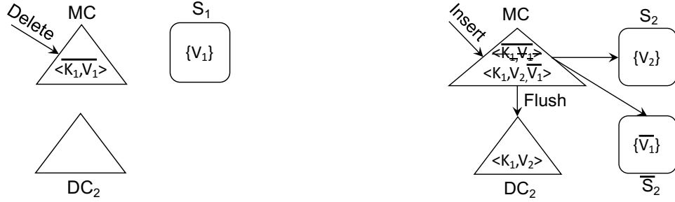
(a) State after deletion of the record R . Value V_1 of the field of a deleted record is a part of the anti-matter record \langle K_1, \bar{V}_1 \rangle along with the key.
