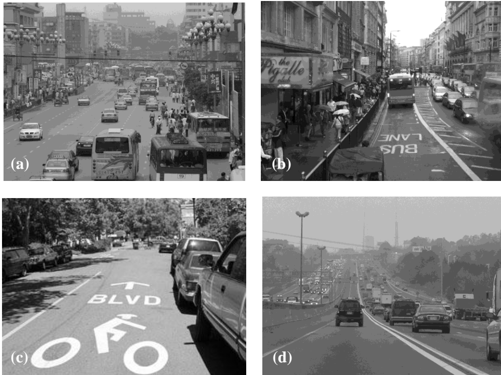
Figure 4. Road space in a multimodal reservoir can be (a) shared by mixed traffic or (b) separated by modes. Space can be dedicated to specific modes such as special-use lanes for (c) bicycles or (d) high-occupancy vehicles. (Photographs Courtesy: (a) Wendy Tau, (b) Cláudia Almeida, (c) ITS Berkeley, (d) Valerie René)
