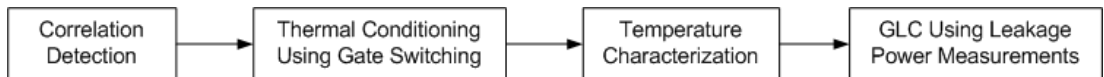
Figure 3.2: Flow of thermal conditioning for GLC. We increase the temperatures of a subset of gates in the circuit to break the correlations in the system of linear equations.
