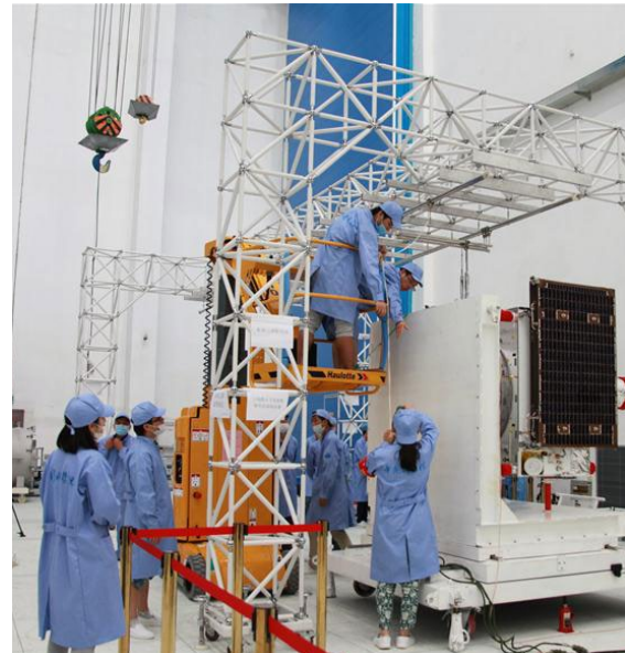
Solar wing deployment testing for quantum satellite Micius . Photo: Xinhua
