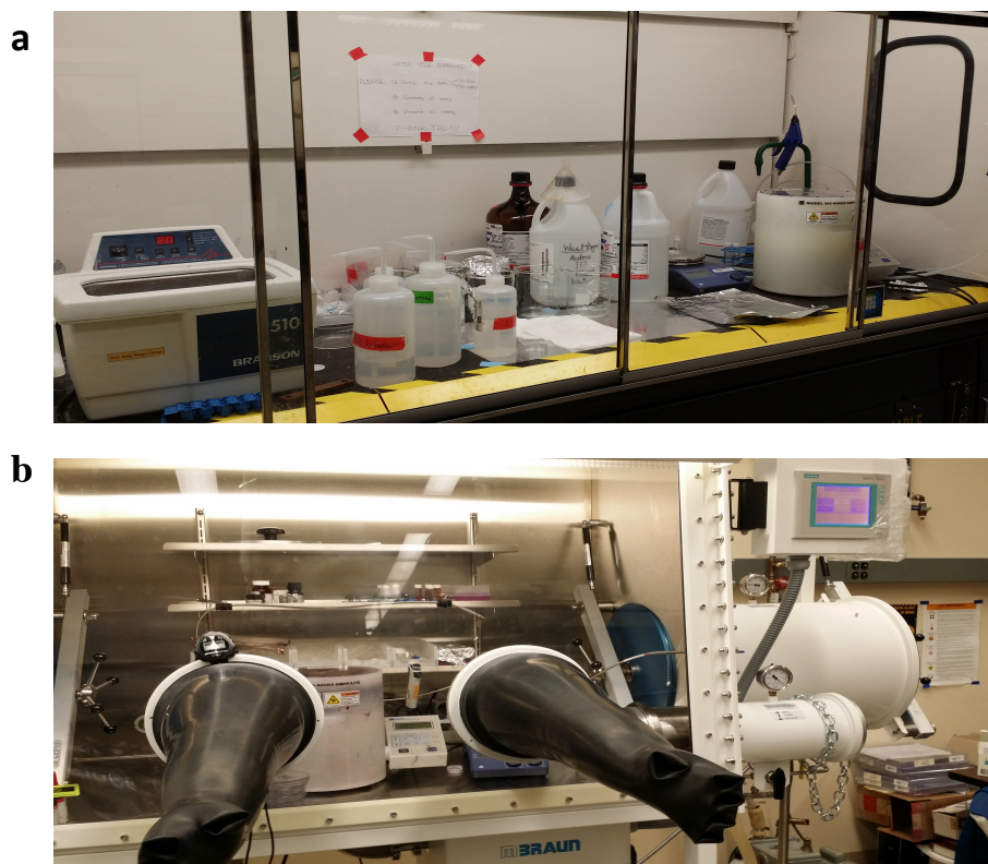
Figure 3.1.1. a) First stage to prepare OPV device, purification and super cleaning of ITO substrate using sonication
