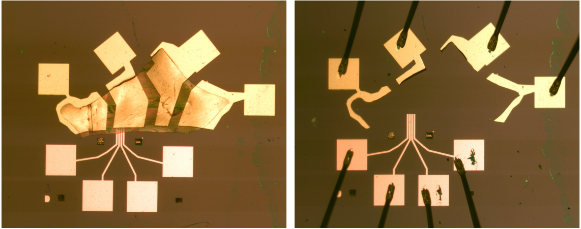
Figure 2.3: Left: Finished diamond flake without a PMMA capping layer. Right: Diamond flake delaminated during electronic measurement.
