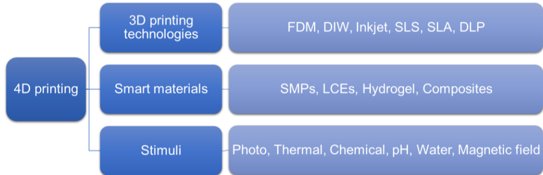
Figure 1.4 Diagrammatic representation of the critical factors of 4D printing.
