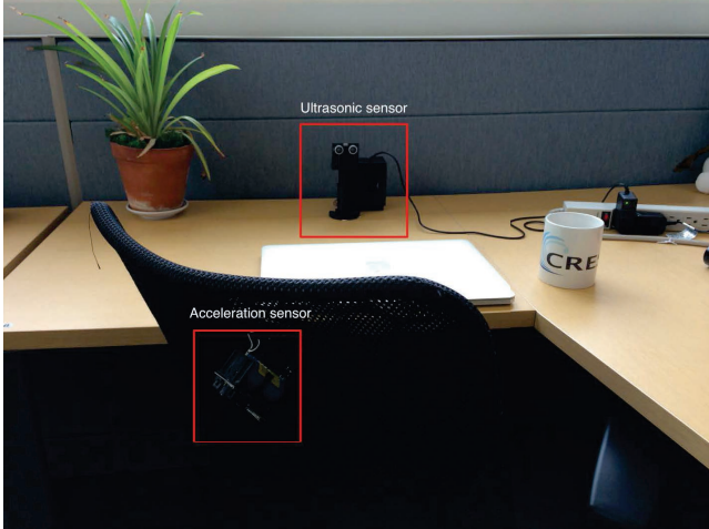
Figure 3. Experimental setup of the ultrasonic sensor and acceleration sensor. The location of the ultrasonic sensor is chosen so that it directly faces the user when he/she is working on the desk, and there should be no obstacles in front of it once the user departs. The acceleration sensor is attached to the chair in order to sense the chair movement. It is very uncommon that users share chairs, so the movement is a unique indicator of presence.
