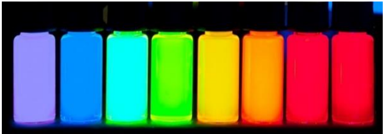
Figure 1.1. Photoluminescence from quantum dot suspensions. Each vial contains a solution of colloidal quantum dots, increasing in size from left to right. (Figure adapted from Antipoff, 2012. CC BY-SA 3.0. Wikimedia Commons).
