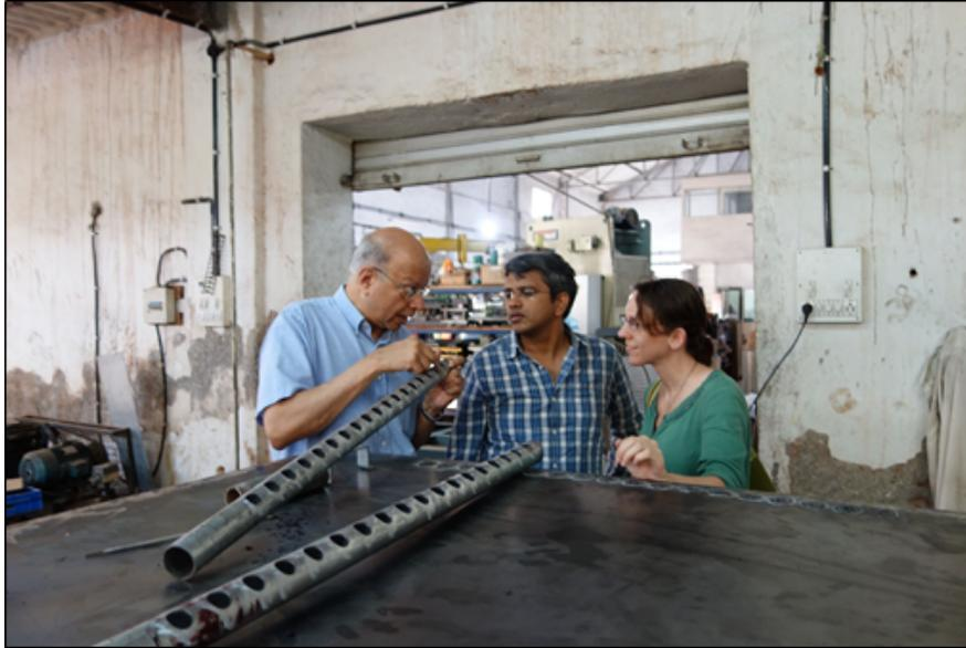
**Fig. 5.3** Ashok Gadgil, Shri Hari Chief Design Engineer, Narendra Shenoy, and Susan Amrose in November 2014, discussing the design details of the water distribution manifold of the two ECAR reactors then under construction.
