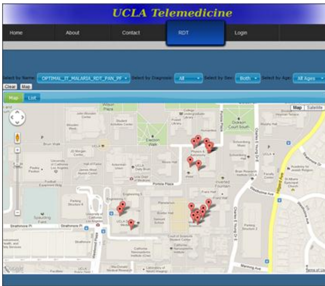
Figure A.4 Web interface of the Real Time RDT Map generated by the central server is shown. This global database stores and organizes test results uploaded by users. The server displays the test data on an internet browser using Google Maps and can filter the data displayed based on several attributes, including: disease type, test location and
