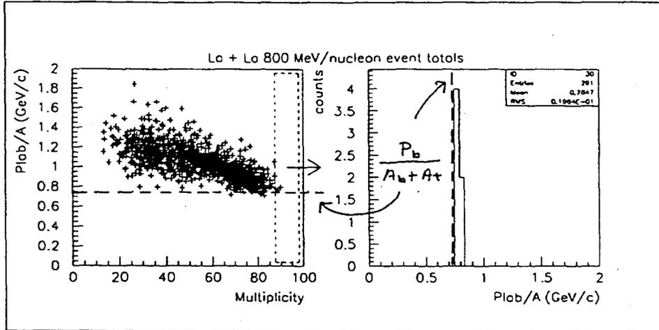
Fig. 5: The measured quantity,  $p_{lab}/A_{measured}$  is shown as a function of multiplicity. The limiting value,  $p_{labbeam}/(A_{beam} + A_{target})$ , that would be seen if all the particles were detected is shown for comparison.
