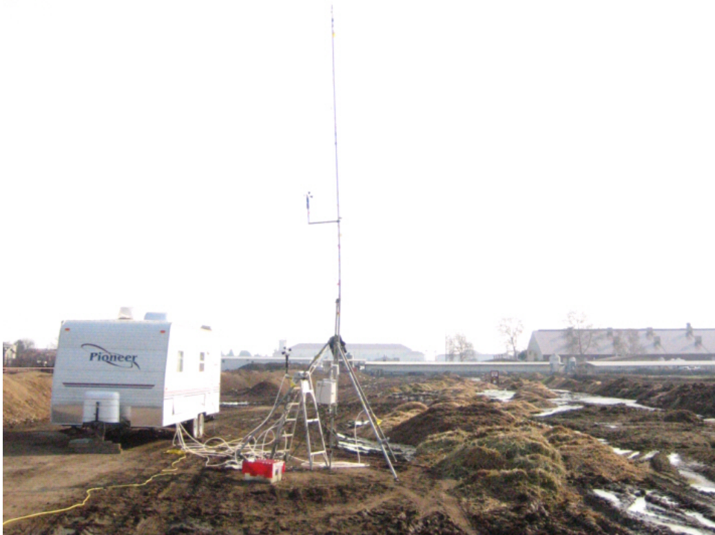
Figure 45: Instrumentation Trailer (left) with Sensor Tower (2/8/08) over the compost pile
