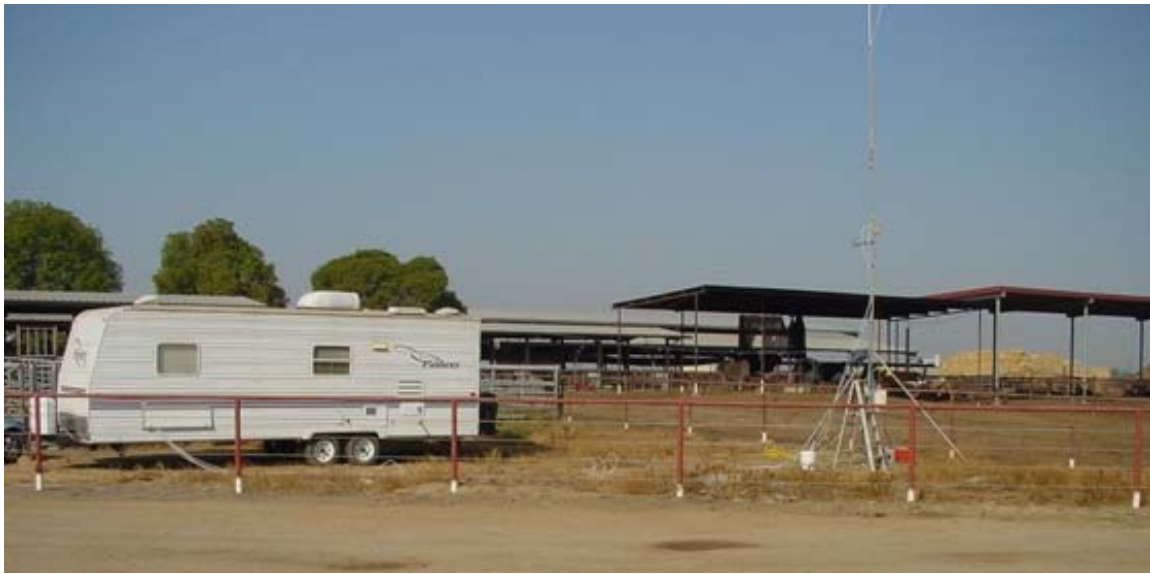
Figure 33: View of site, photo taken from the southeast. It shows the relationship of the tower to the trailer, and the five meter gas sampling point can also be seen.
