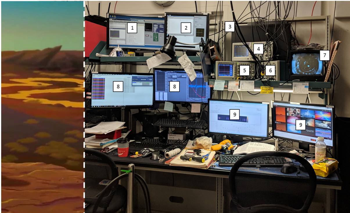
Figure L.4: 1: Rivers monitor. 2: TARTH monitor. 3: Rivers (control computer for 403 nm digital lock to cavity signal, scope traces from Kapitza-Dirac diffraction). 4: Monitor for lattice PIDs. 5: Monitor for ODT/XODT PIDs. 6: Monitor for MOT currents, 689 nm MOT PID. 7: MOT fluorescence camera monitor. 8: Arryn monitors. 9: Blackfyre monitors. Left: “What about that shadowy place?” “That’s beyond our borders. You must never go there.”
