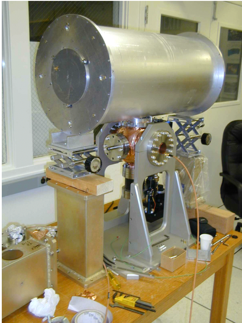
Figure 98. ALS third harmonic cavity with energy storage cavity.
