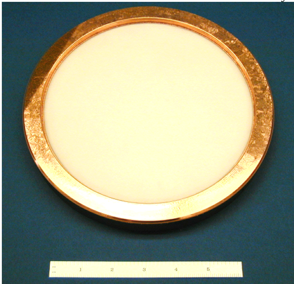
Figure 56. Window #2 as brazed.
