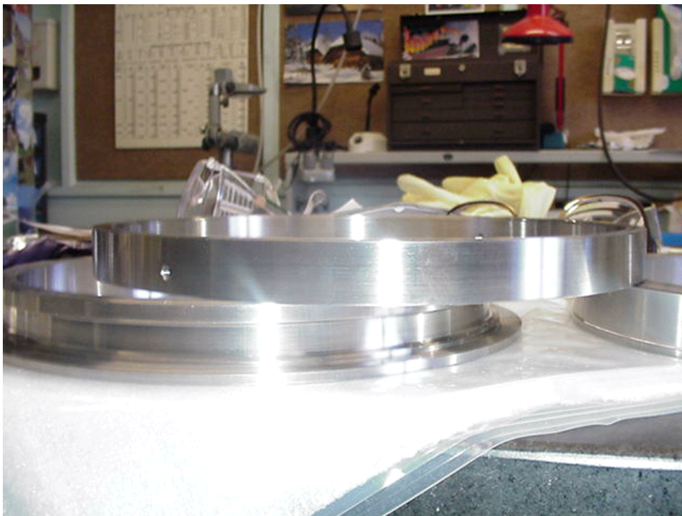
Figure 52. Hollow cooling ring parts ready for brazing.
