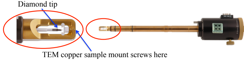
Figure 3.10: PicoIndenter PI95 holder for in situ TEM uniaxial compression test
