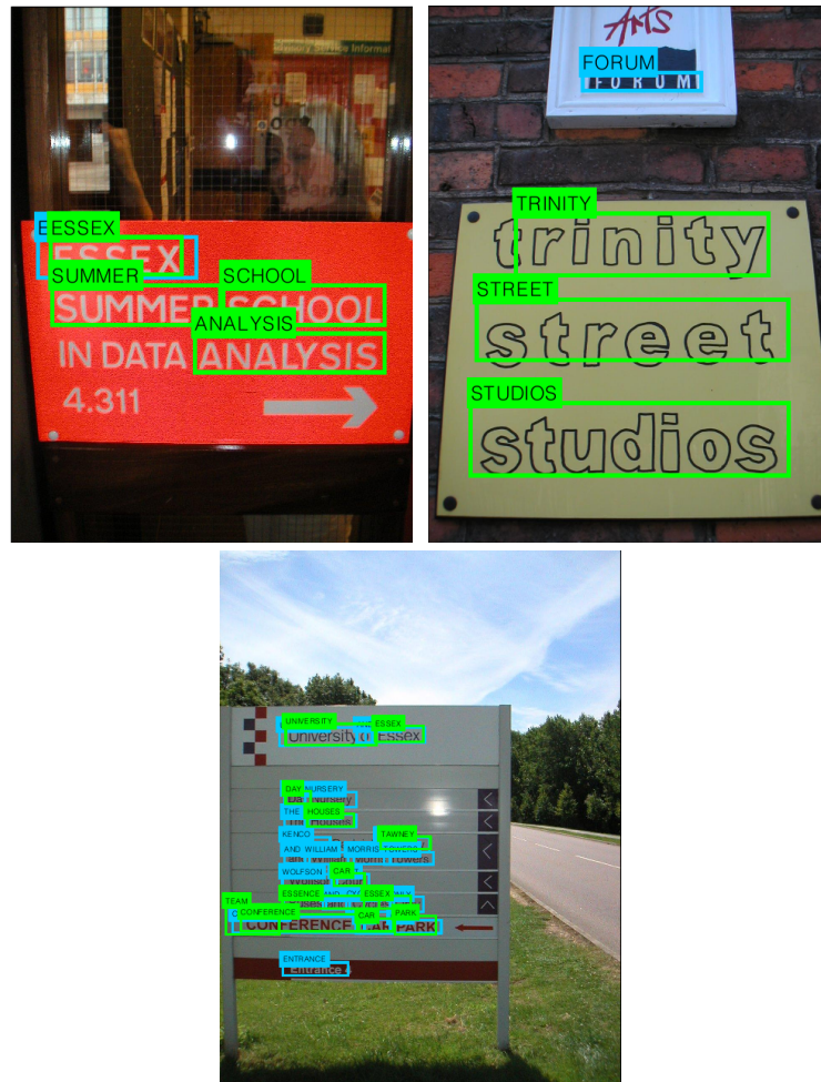
Figure 4.8: Selected results of end-to-end methods on the ICDAR dataset (for a lexicon with K = 20 distractors). Results from PLEX+R are shown in green and results from SWT+ABBY are shown in blue. In the first two images ABBYY has trouble reading text with noisy image conditions and unusual fonts; the last image is more well suited for ABBYY as it is more similar to a scanned document.
