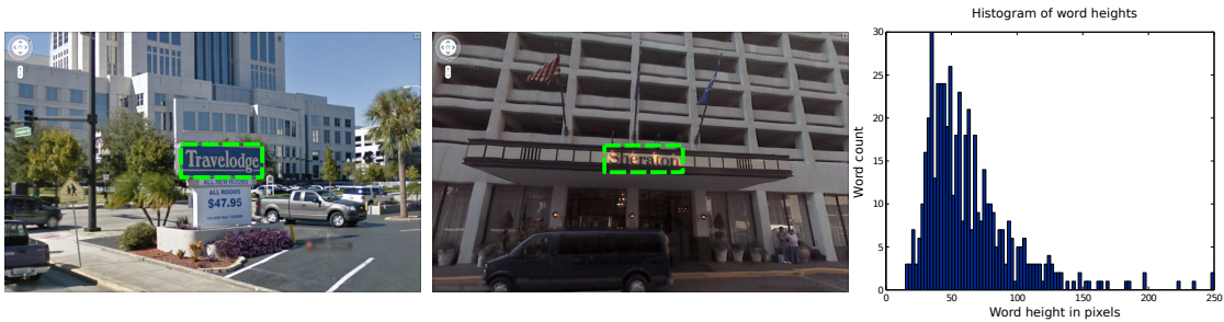
Figure 2.1: Examples from our Street View Text (SVT) data set and a histogram of word heights. The words appearing in this data set have high variability in appearance, suffer effects of cast shadows, and often have low resolution. The median height is 55 pixels.
