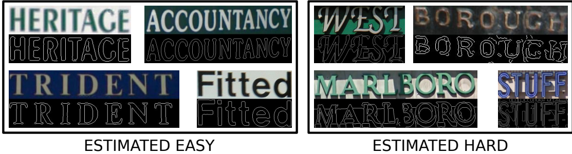
Figure 3.4: In our analysis, we use a simple and intuitive heuristic based on edge detection to group images into EASY and HARD. The EASY examples are typically those whose characters are well outlined, and the HARD ones typically contain more broken characters and edges from the background and shadows. This is a coarse estimate of those images that are more CAPTCHA-like.
