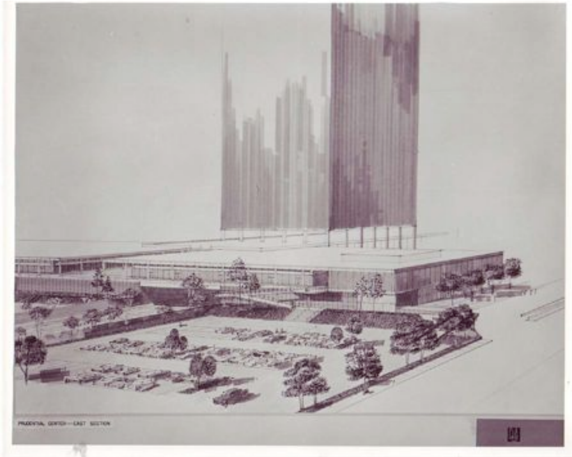
Figure 5.20. CLA produced a rendering of the landscaped parking lot that would occupy the eastern section of the Prudential Center site. Note the uncovered portion of the Mass Pike extension that would cut through the surface parking lot. Source: PA 17-68.
