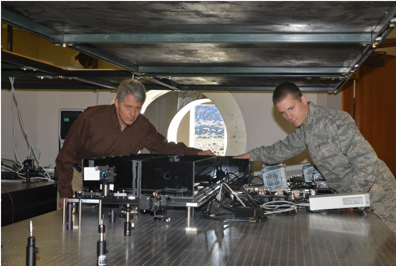
Figure 7.5. In 2019, Air Force Research Laboratory scientists demonstrated daylight QKD using this rig at the Starfire Optical Range, located at Kirtland Air Force Base in Albuquerque, New Mexico. This is important because stray daylight entering the collector causes substantial noise that interferes with the measurement, limiting long-distance QKD during the daytime. (The Air Force’s Directed Energy Directorate, which develops lasers and optics, was identified for transfer to the US Space Force in 2020.) Image by US Air Force photographer Todd Berenger.
