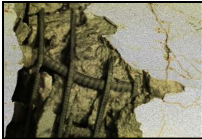
Figure 7-2. Close-up of surface mesh of failed structural specimen with overlaid texture map.
