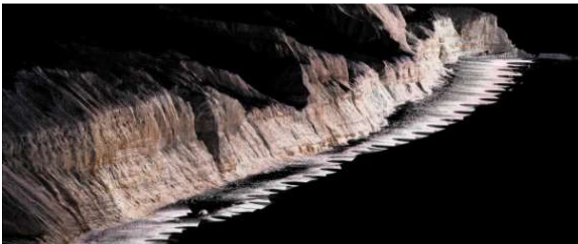
Figure 2-2. Georeferenced point clouds for regional mapping of Torrey Pines, CA (September 2007). Black semi-circles represent scan setup locations spaced at approximately 50 m.
