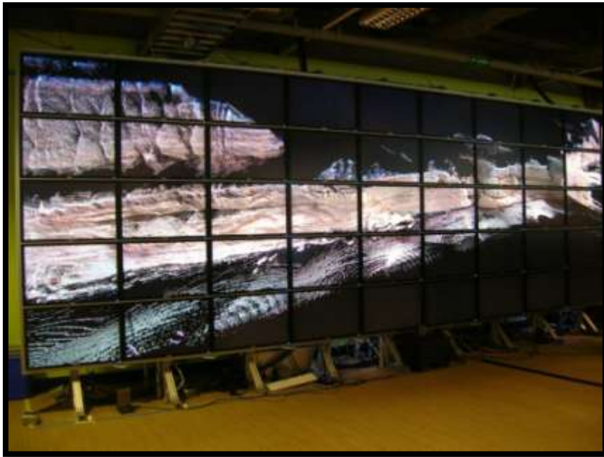
Figure 7-6. Display of coastal dataset on Hiperspace tile display wall, a 286 Million Pixel Display
