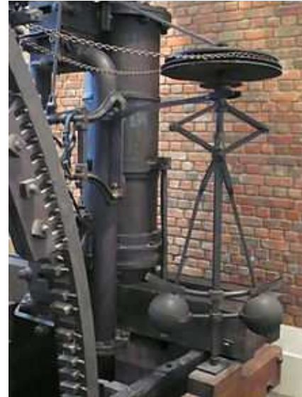
(b) Watt's centrifugal governor.
