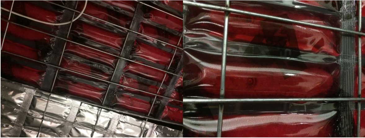
FIGURE 22 : ROUND 1 (TOP) AIR TEMPERATURE IN THE PLENUM ON 07/06, (BOTTOM) PICTURES OF THE CLEAR PACKAGE PCM TAKEN ON 07/06 5PM PST (CAV -5)
