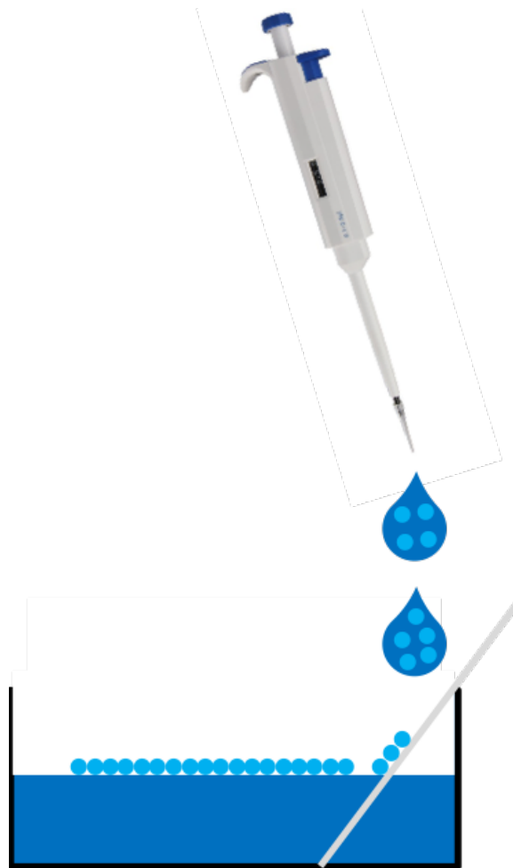
Figure 1.7. Experimental setup to prepare high-quality polystyrene monolayers via the Langmuir-Blodgett method.
