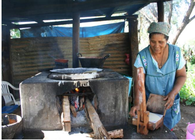
Doña Simona works on her fogón ; her husband built it in their space behind their home, it is surrounded by their traspatio where she obtains fresh ingredients for her cooking. This fogón is protected by a roof and two walls. Photograph taken by Armando Quiroz.
