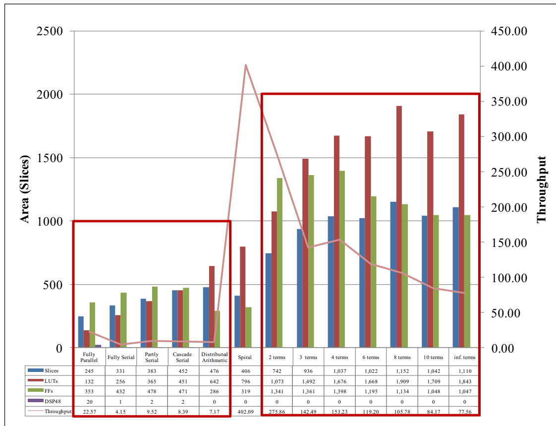
Figure 3.10: Comparison of Xquasher, Spiral and Filter Design HDL Coder Toolbox architectural results for 20 tap FIR filter designs. Different architectures designed using Design HDL Coder Toolbox include fully parallel, fully serial, partly serial, cascade serial and distributed arithmetic. Xquasher performs different number of term extraction: 2, 3, 4, 6, 8, 10 and infinite terms to find most suitable extraction method that provides best results in terms of area and throughput.
