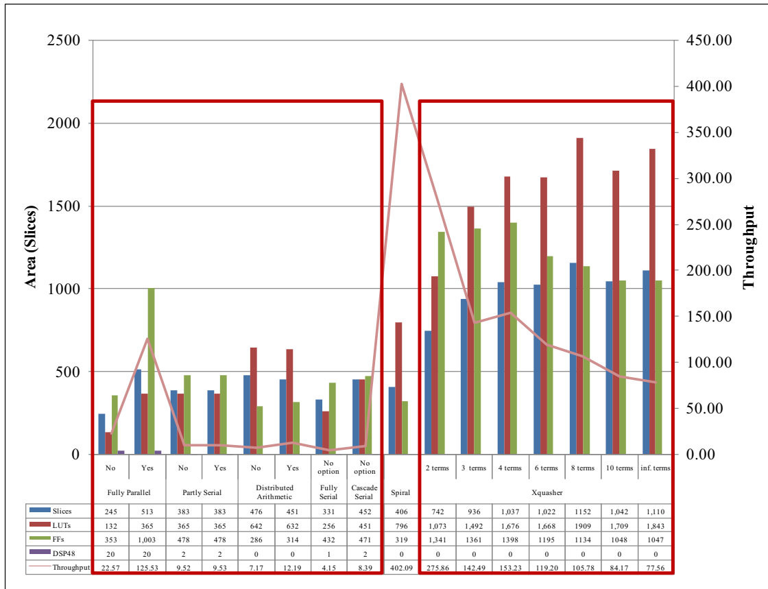
Figure 3.14: Comparison of Xquasher, Spiral and Filter Design HDL Coder Toolbox architectural results for 20 tap FIR filter designs that includes an option for use of pipeline registers for Filter Design HDL Coder Toolbox. Different architectures designed using Design HDL Coder Toolbox include fully parallel (with and without pipeline registers), fully serial, partly serial (with and without pipeline registers), cascade serial and distributed arithmetic (with and without pipeline registers). Xquasher performs different number of term extraction: 2, 3, 4, 6, 8, 10 and infinite terms to find most suitable extraction method that provides best results in terms of area and throughput.
