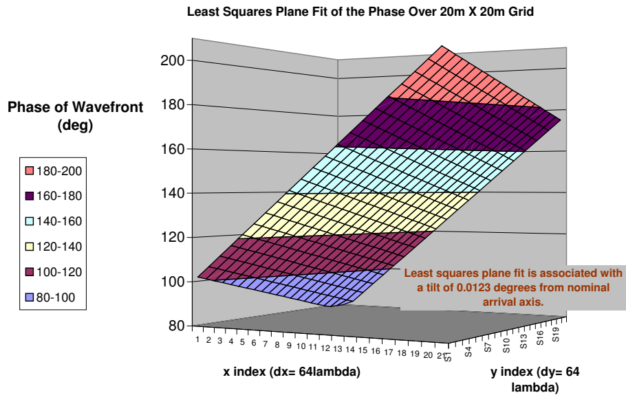
Figure 1.9: The least squares fit to the example phase front.
