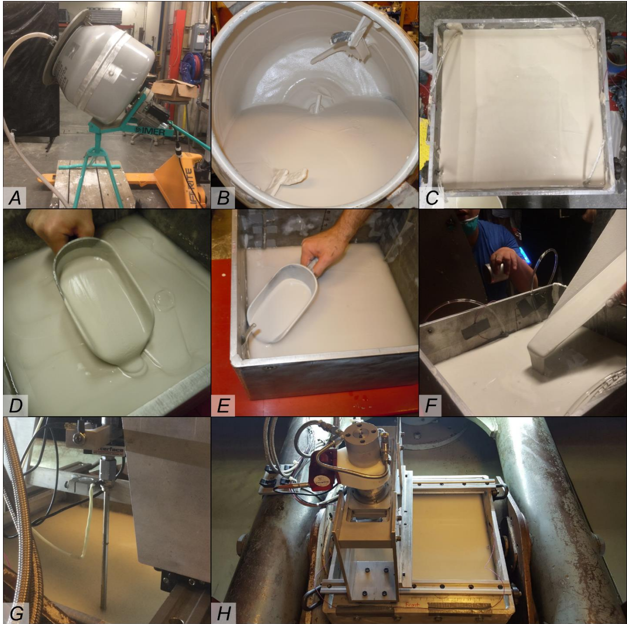
Fig. 6. Centrifuge model construction: (a) vacuum slurry mixer; (b) mixed 97.5S2.5K slurry; (c) pre-consolidated 80S20K model; (d) slurry deposition of the 97.5S2.5K mixture; (e) slurry deposition of the 95S5K mixture; (f) slurry deposition of 100S silt; (g) 6-mm cone penetrometer and actuator rack; (h) silt model with cone actuator rack on 1-m radius centrifuge
