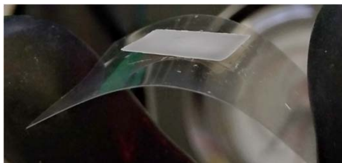
Figure 2.13. To demonstrate the robustness of SSE films selected from class 1, a free-standing SSE film was cast on a PET film and vacuum dried. After calendaring, the SSE film can be peeled from the PET film without any damage.
