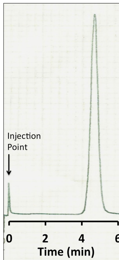
Fig. 1 Gas chromatography analysis of isoprene (2-methyl-1,3-butadiene; C 5 H 8 ) standard. One milliliter of a vaporized isoprene sample comprising 0.087 μg pure isoprene was injected into the column inlet of the GC. The retention time for isoprene under these GC conditions was 4.3 min. Samples collected from the headspace of experimental cultures were similarly analyzed from their single peak amplitudes at 4.3 min
