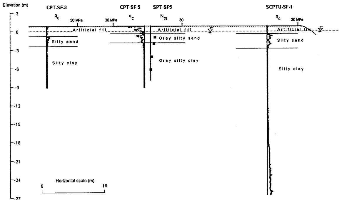
Fig. 8. Cross section I-I of soccer field site
