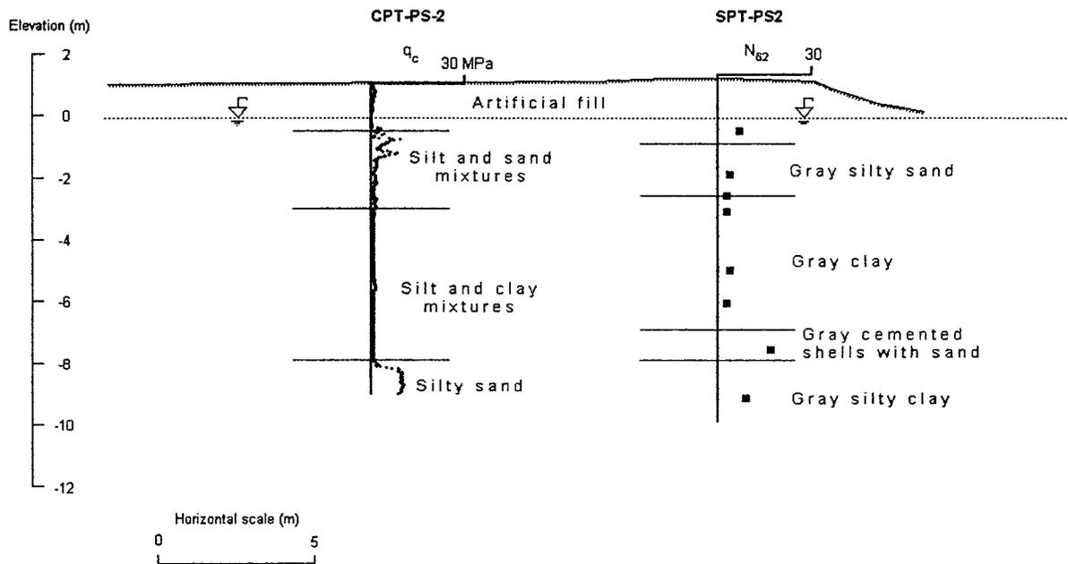
Fig. 5. Cross section II-II of police station site
