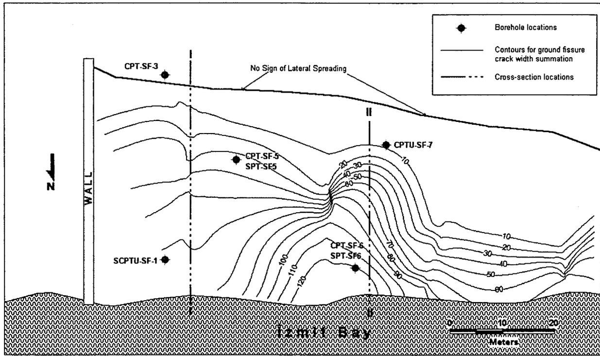
Fig. 7. Ground displacement map of soccer field site
