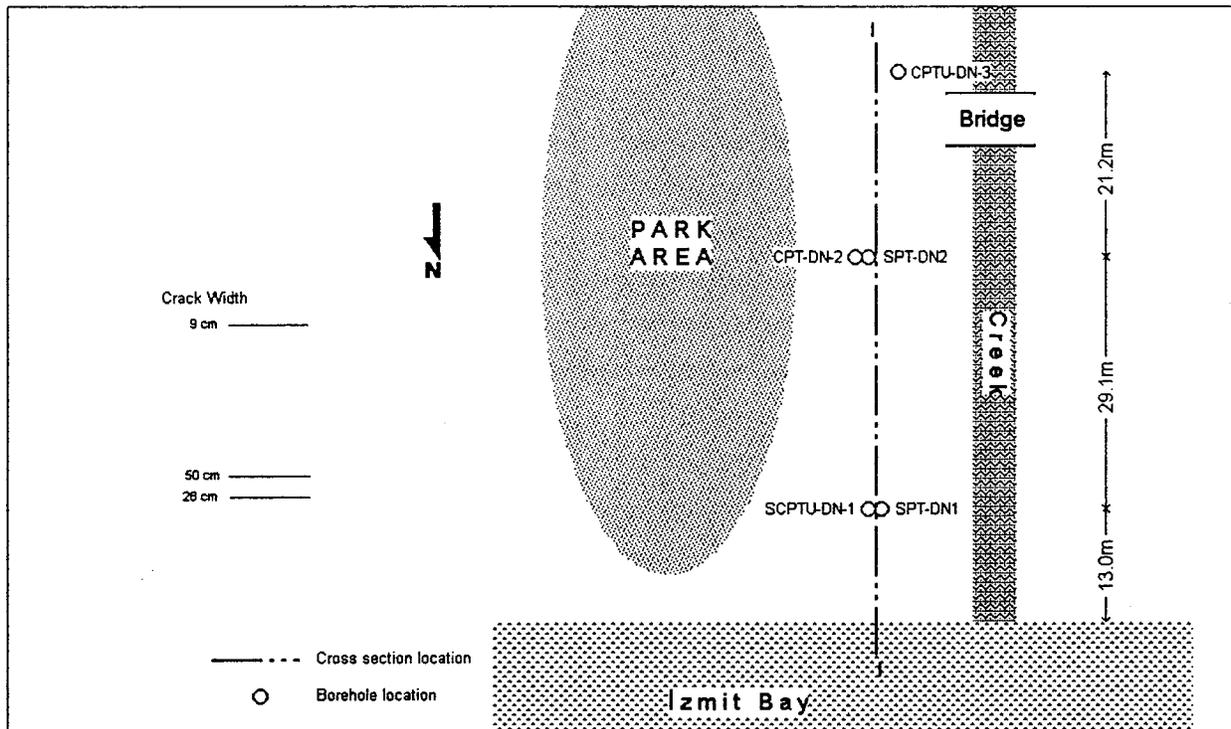
Fig. 10. Ground displacement map of Degirmendere Nose site
