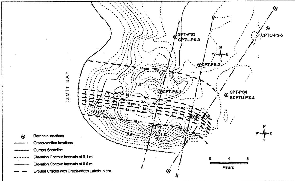
Fig. 3. Ground displacement map of police station site
