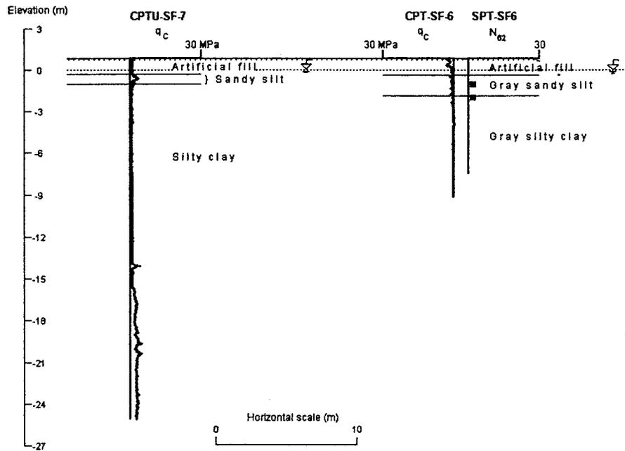
Fig. 9. Cross section II-II of soccer field site
