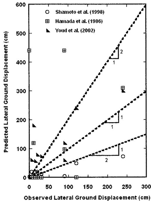
**Fig. 15.** Comparison of predicted versus observed lateral spreading displacements
