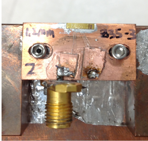
Figure 4.1: Top view of a Z35 device successfully mounted on a copper submount.
