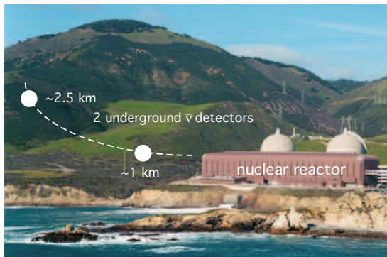
Figure 2. Concept of a 2-detector neutrino oscillation experiment at the Diablo Canyon nuclear power plant in California.
